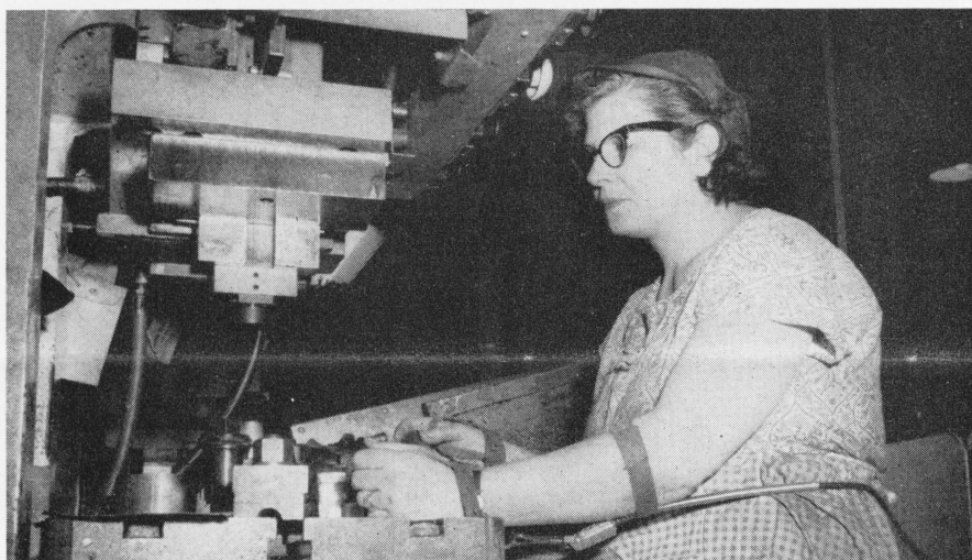
Angeline Maiette, Press 2, found that the wrist safety bands stretched and were therefore useless. She devised a new band, made up a sample, tried it and then turned in the suggestion. It is now in the hands of the Purchasing Department to be procured for use wherever necessary.
